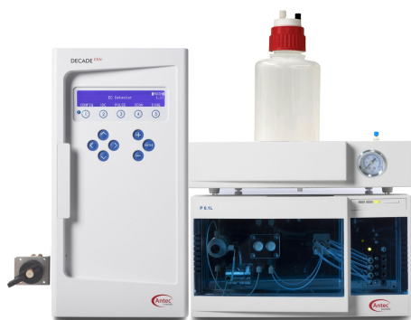
Figure 5. Dedicated ALEXYS FDG analyzer consisting of a DECADE Elite with SenCell Au- HyREF, P 6.1L isocratic pump, ET 210 eluent tray, manual injector and Clarity CDS for instrument control and acquisition.
